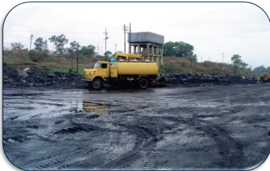
FIGURE 4.13 WATER TANKER FOR SUPPRESSION OF COAL DUST
