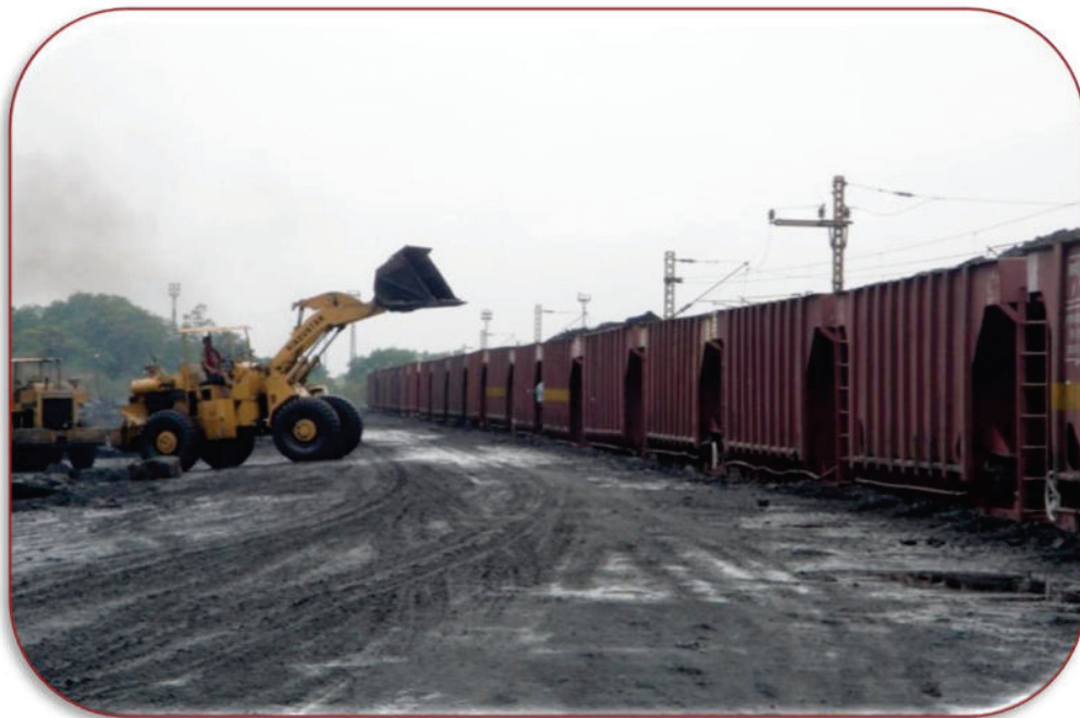
FIGURE 4.1 LOADING OF COAL THROUGH JCB
